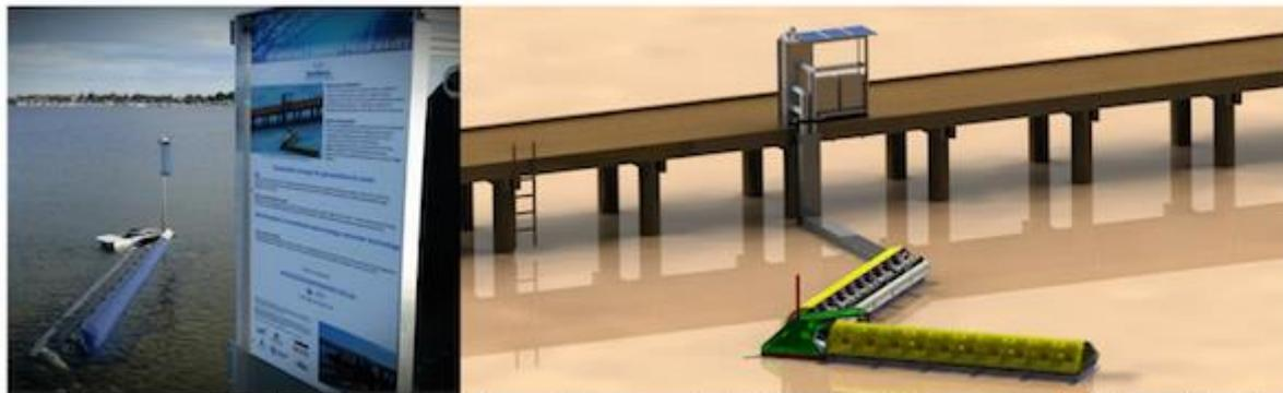
L. Bombora mid-scale prototype (affectionately known as Karl) deployed in Melville waters. R. CAD graphic of the deployment.
