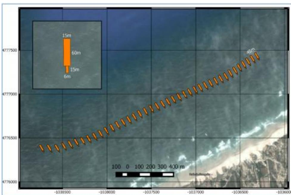
Figure 1: Bombora's 60MW Wave Farm configuration
