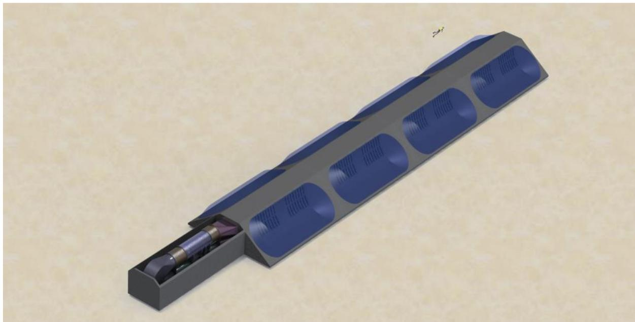
Figure 2 – Bombora's 1.5MW mWave Wave Energy Converter
