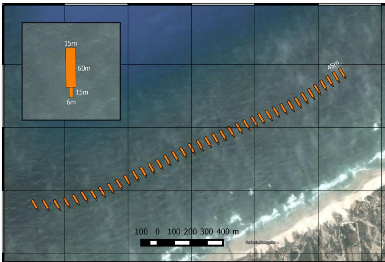
Figure 1 – Bombora's 60MW mWave Farm Configuration
