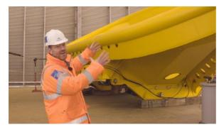
Bombora's Chief Operating Officer Dave Rigg leads the Assembly Centre tour stopping to explain how the innovative mWave cell module will be covered in a flexible rubber membrane
